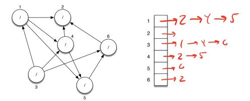
(b) Perform a DFS using vertex 4 as the source. (For any new trees, start at the smallest available vertex index).
