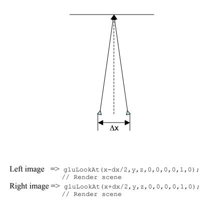
This method, while simple, produces vertical parallax issues (come discuss it with me for more details). A better method is known as parallel parallax which has the two cameras pointing in the same parallel direction. This would be done using
