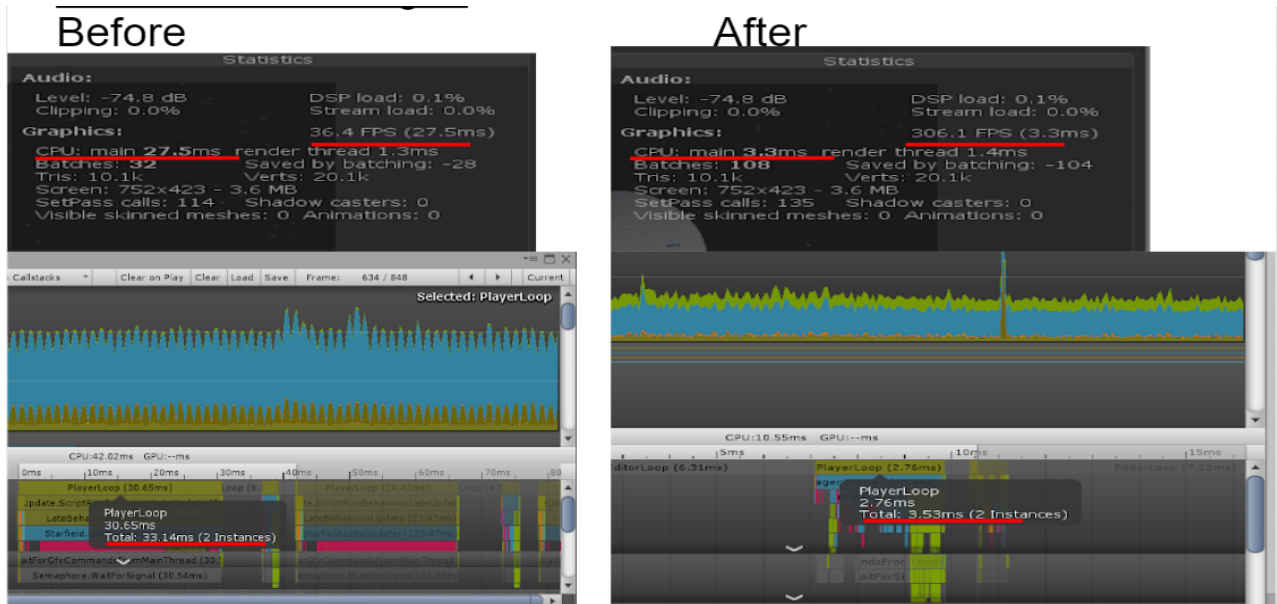
Figure 5: Unity profiler view of before and after “Starfield” script fix. (grass was disabled)
