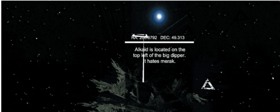
Figure 15: VR controller with line renderer indicator, selection of star object is shown.
