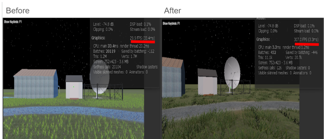
Figure 7: Before and after visualization of the new grass model and new pavement terrain texture. Notably the frametime improved from 33.4ms to 3.3ms. Notably, the triangle count of the program reduced from 1.2 million triangles to a measly 11.1k triangles, which is fantastic.
