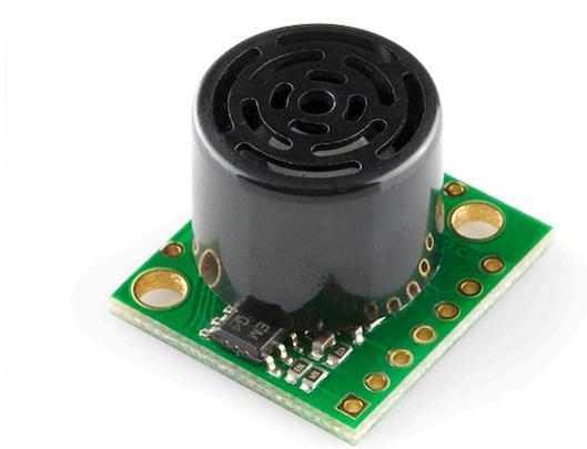
**What It Does:** The range finder sends out pulse of ultrasonic (inaudible) sound and listens for reflections. Based upon how long it takes for the pulse to return, the sensor can roughly measure distance.
