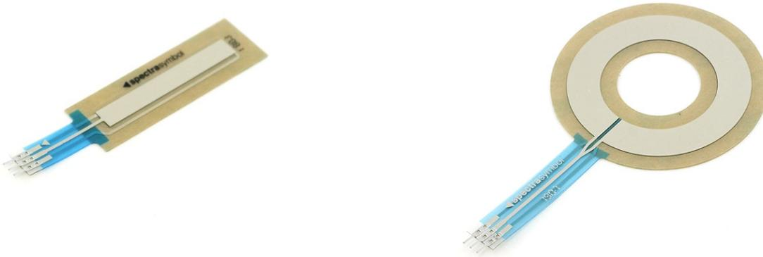
**What It Does:** Each slider is a variable resistor that changes its value when touched. The resistance changes linearly over the length of the sensor, so we can determine exactly where it's being touched.
