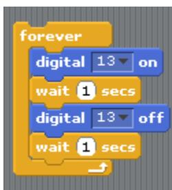
Figure 3: Turn the Motor On and Off Every Second
