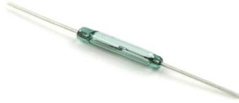
**What It Does:** A reed switch is two pieces of metal that touch when a magnet is nearby. Normally they are separated and no electricity can pass.
