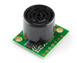
**What It Does**: The range finder sends out pulse of ultrasonic (inaudible) sound and listens for reflections. Based upon how long it takes for the pulse to return, the sensor can roughly measure distance.
