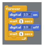
Figure 3: Turn the Motor On and Off Every Second
